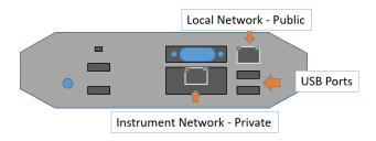
This port is intended for local network access with the firewall configuration included as Public. The second RJ-45 port uses the IO Expansion interface with the connector located in the cutout to the left of the USB ports. This port is configured as Private in the firewall and must be used for the connection to the instrument. In the following two illustrations, the first one shows the Ethernet connections and the second shows the Windows firewall.
